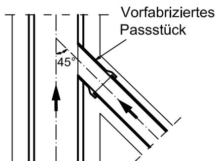
Anschluss an Kanal in Beton/Stahlbeton/
